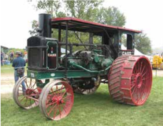
A fine old example of an early Case gas/oil two-cylinder tractor, circa, 1916.
